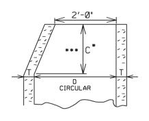
THE CONE OF THE VALVE VAULT SHALL BE CONSTRUCTED AS SHOWN ABOVE ONLY WHEN THERE IS INTERFERENCE WITH UNDERGROUND CONDITIONS AND THOSE CONDITIONS CANNOT BE ALTERED, OR WHEN THE OFFSET IS REQUIRED TO CENTER THE VALVE OPERATING NUT IN THE OPENING.
