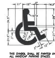
HANDICAP PAVEMENT MARKING DETAIL
