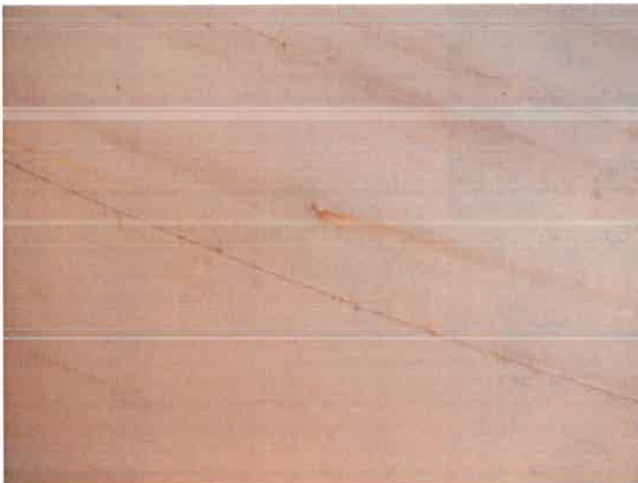
45) Spot coating failure with rust undercutting on the bowl.
