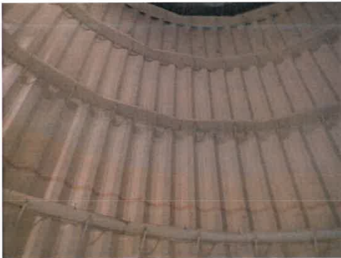
37) The column coating above the condensate platform is in good condition overall.
