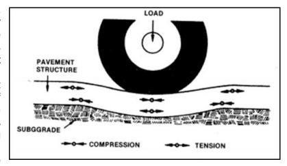
cracks weakening the subgrade. A weakened subgrade susceptible to moisture speeds-up the deterioration cycle to a point when the only recourse is reconstruction. Moisture and oversized vehicles are the key factors in pavement fatigue.
